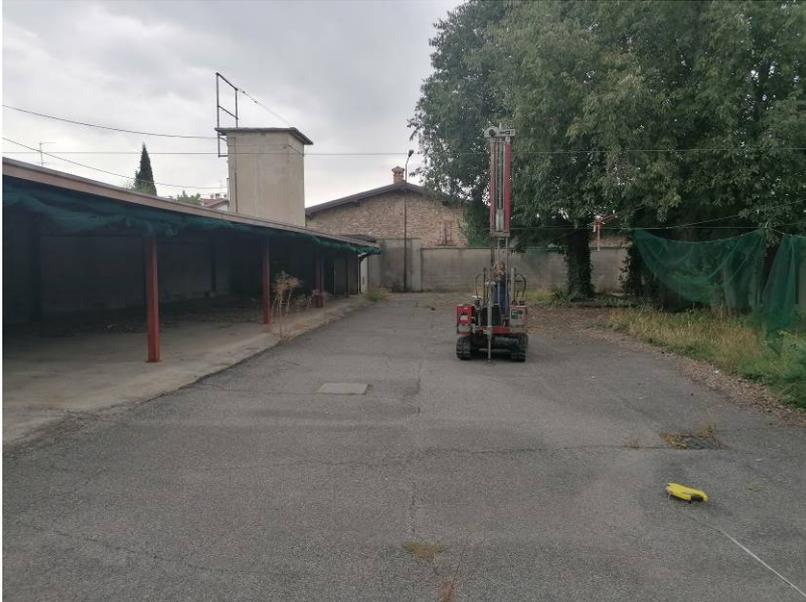
Fig. 17 Prova penetrometrica SCPT
